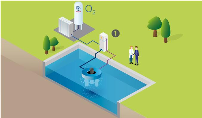
Installed with an OXY INJECTOR-TURBOXAL
